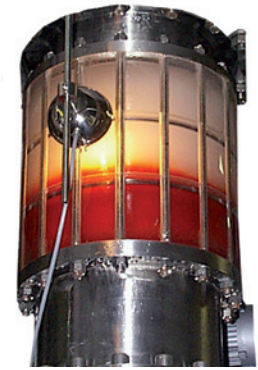
Wash column with wash front
