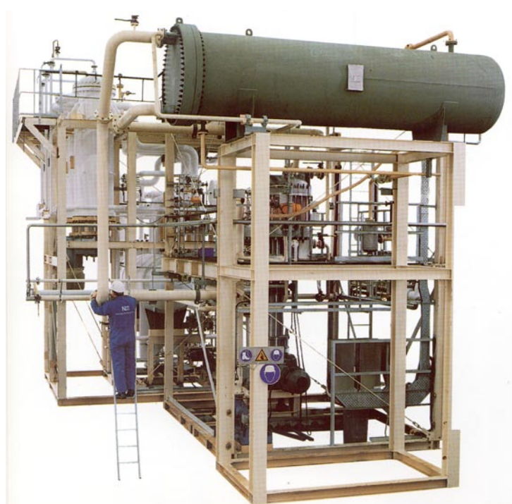
Waste Water Concentration Plant
