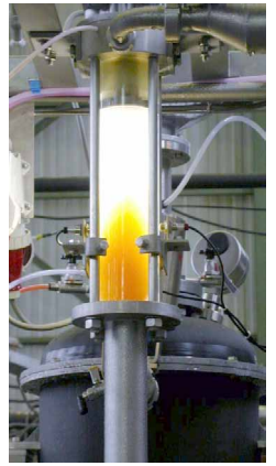
W6 wash column illustrating the sharp separation between the washed ice crystals on the top and those still surrounded by concentrated product on the bottom.
