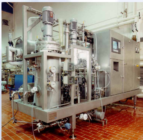
Commercial configuration for the NFC-W6, a stand-alone freeze concentration unit complete with refrigeration and control system.
