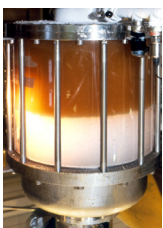
The sharp separation between the washed and unwashed portion of the crystal bed (wash front) is illustrated on a W60 screw-type wash column.
