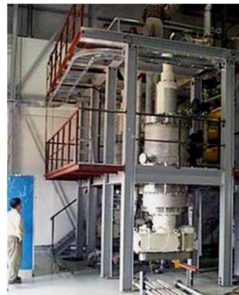
Melt crystallization plant for production of electronic grade phosphoric acid
