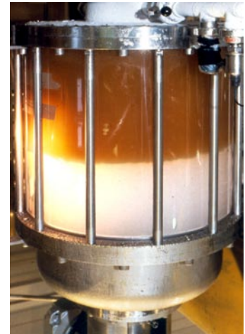
The sharp separation between the washed and unwashed portion of the crystal bed is illustrated in a wash column with transparent cylinder.
